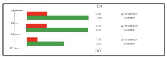
3.) Time control and Sensor control: as per below(can be customized)
